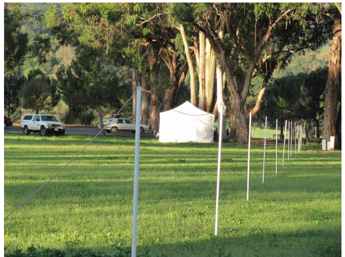
Beverage Antenna for receive on 160-Meters
